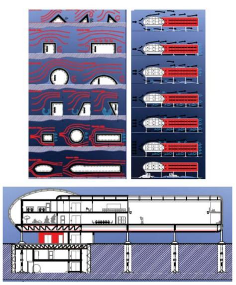
Figure 6: A study of aerodynamics of forms and the resulting solution for an Antarctic energy-effective station (Source: P. Duda and R. Kalinowski, *Diploma design*) [5].
