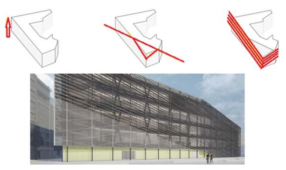
Figure 4: Form-finding analysis of an office building based on a study of insolation and its final shape (Source: A. Dziewit, *Diploma design*) [5].
