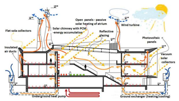
Figure 3: An energy diagram of a building with the close to zero demand for non-renewable primary energy. The building as a system of interrelated solutions. Research and educational complex of the Faculty of Environmental Engineering, Wrocław University of Technology (Source: P. Kuczia, *Educating Buildings*) [4].
